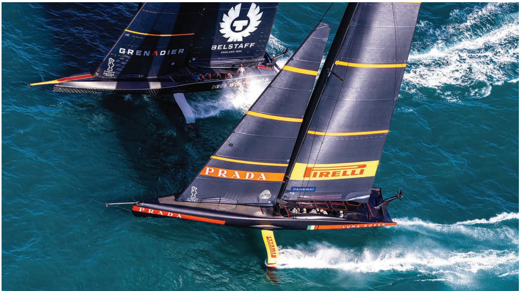
Today's sails are molded with carbon fiber on forms. Change inspired by the 1983 America's Cup loss have lead to boats that are five times faster than any sailing vessel on the water in 1983
